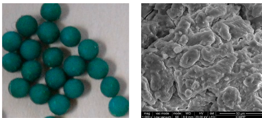
Figure 9. Optical (left) and SEM images (mag. 1000×) (right) of the composite CS 80 AOX 20 -A.2 loaded with Cu 2+ .
